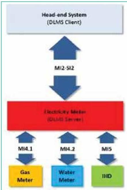
Figure 5. FID-2 package 1 system architecture
