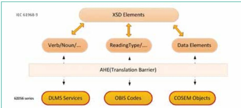
Figure 4. One-to-one correspondences between IEC 61968-9 (upstream) and DLMS/COSEM (downstream).
