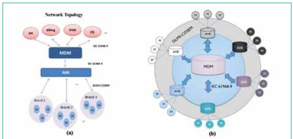
**Figure 2. Interoperability concept in IRAN smart metering project (high-consumption customer).**
