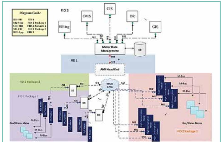
**Figure 1. The smart metering project's information exchange architecture (conceptual architecture of FAHAM interoperability between smart meters, AHEs, MDM, and application systems).**
